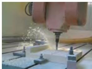
CNC-milling of a lightweight PUR board.
