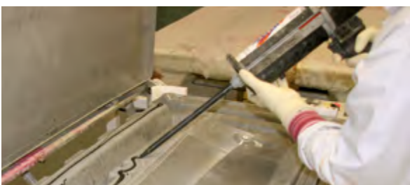
Bonding of SMC parts with Adekit A280.
